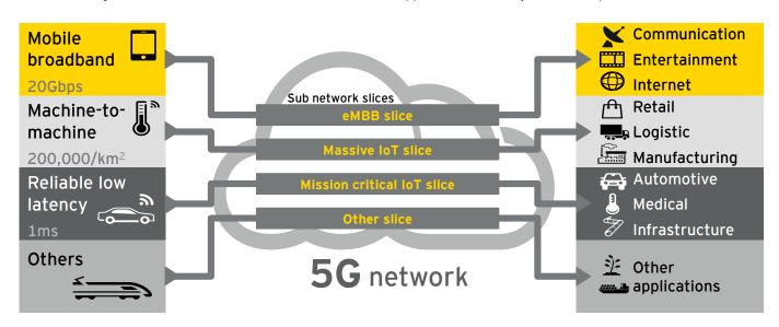
Network slicing subdivides 5G network into virtual slices to tailor applications with very different requirements
