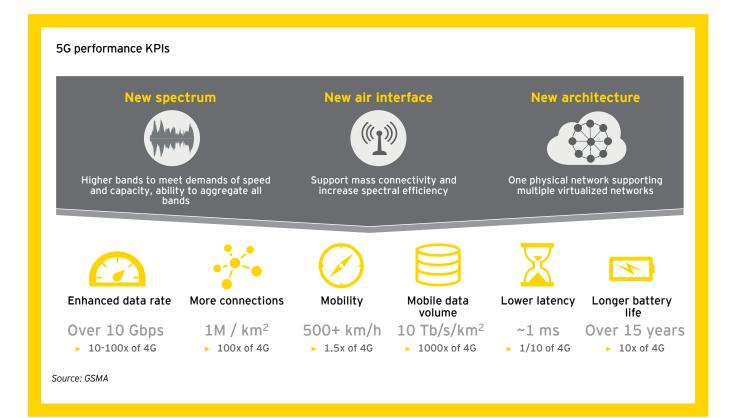
The disruptive capabilities of 5G will pave the way for new innovative applications that the current LTE technology cannot support. Some of the widely promoted examples include industrial automation and utility services, vehicle-to-vehicle and vehicle-to-infrastructure transportation, home automation, augmented reality (AR), virtual reality (VR) and many more.
