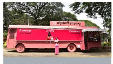
As featured in the joint report with the Toilet Board Coalition, Make way for the future of sanitation (pdf), 3S is repurposing old city buses as sanitation kiosks, complete with toilets, shower cubicles, diaper changing stations and sanitary pad vending machines. These provide a safe, clean and familiar sanitation experience for low-income urban women in Pune, India. Photo courtesy of 3S.
