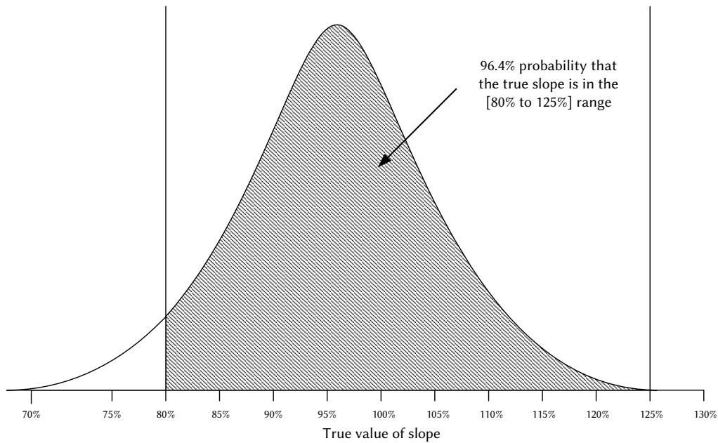
Figure 52.3: The probability distribution of the true slope, for the given sample, follows a t -distribution, with a 96.4% probability that the slope is within the 80% to 125% range
