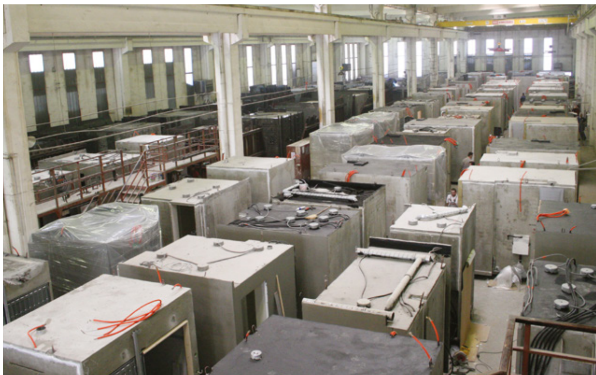
Their prefabricated bathrooms, made from lightweight concrete are separate construction elements, delivered to the facility fully completed
