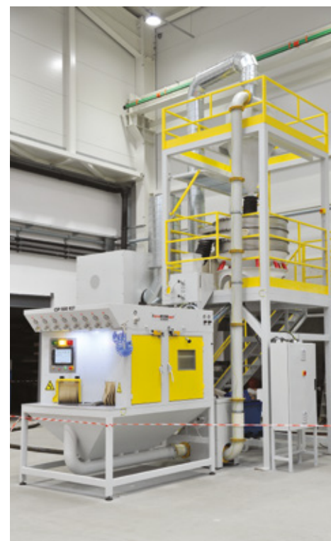
Machine for shot peening of jet engine blades
