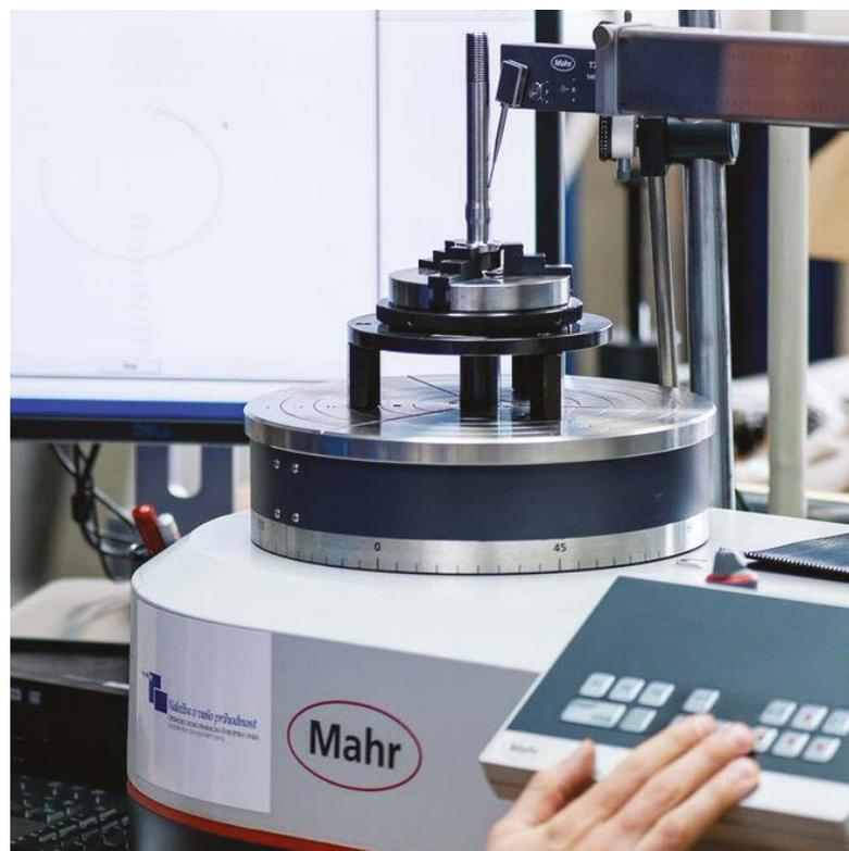
Checking dimensions and positional tolerances using the MAHR measuring device
