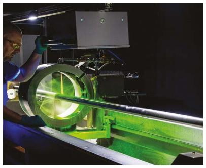
Surface defect control machine - up to 4,000 mm in length
