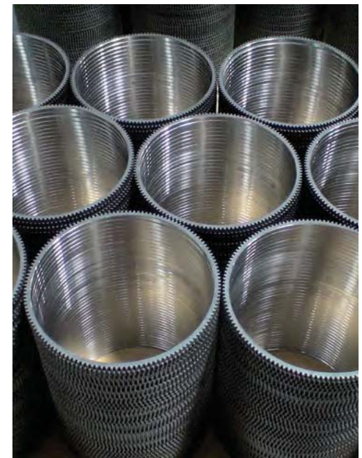
They specialize in the production of ring gears for the automotive industry
